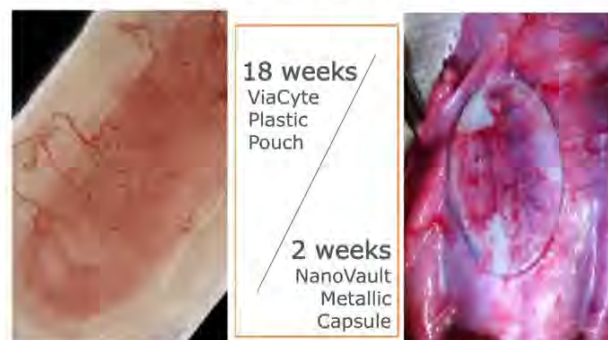
Fig. 2: In vivo increased new blood vessel formation surrounding through-porous nanometals. ViaCyte is an FDA approved polymer stem cell delivery device.
