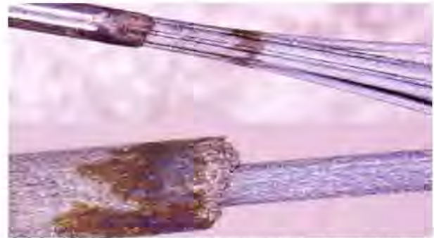
Figure 2. 0.25 mm FeMnN-Mo wires Fig. 1c (top) and Fig. 1f (bottom) shown after partial degradation.
