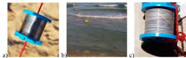
Fig. 1: MgZnCa wire before (a), during (b) & after corrosion (c).
