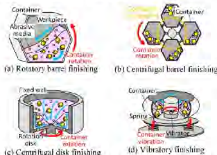
Figure 1: Processes for surface modification using barrel finishing [1]
