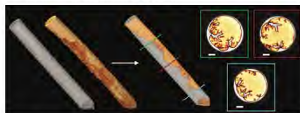
Fig. 1: MicroCT-based images of degradation behavior of Zn alloy. Grey at time point 0 and orange after 7d of immersion. Scalebar = 50 \mu\text{m} .
