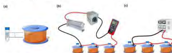
Fig. 1: Experimental set-up (a) Sample in the tube and the cylindrical copper coil (b) H AC configuration. Coils connected to an autotransformer (c) H DC configuration. Coils connected to a DC power supply.
